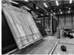
Butterfly table 출처 : Modular Building Automation
